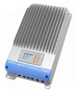
iTracer-ND is an intelligent, efficient ,high-speed solar charge controller with advanced Maximum Power Point Tracking (MPPT) algorithm, which can harvest the maximum power from the solar array to charge battery. It can be applied in the off-grid PV systems up to 3KW, and increase the efficiency up to 30%.
